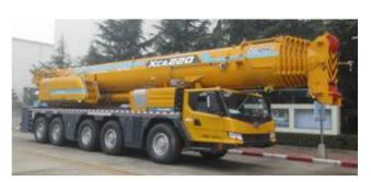
five-axle chassis specialized for all terrain crane, which features better ride-ability, manoeuver ability and pass-ability. Integration of mechatronics and hydraulic system for precise full-axle steering and braking technology contribute to superior ride-ability.
